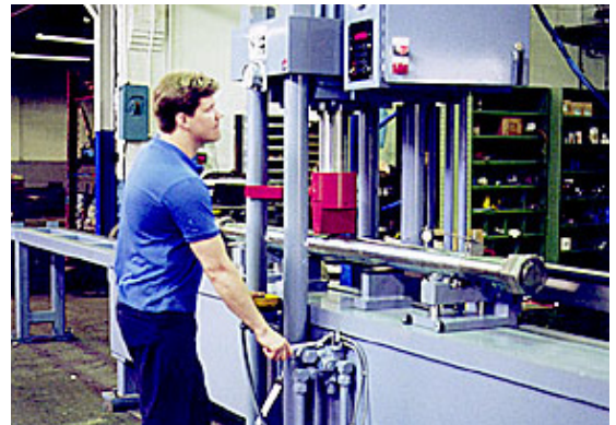
Fixed Frame Straightening Press - 100 ton model with 10 ft. bed and (2) 12 ft. extension tables. Designed for lighter weight bars. The work is loaded onto carriages which are then manually rolled under the ram.
