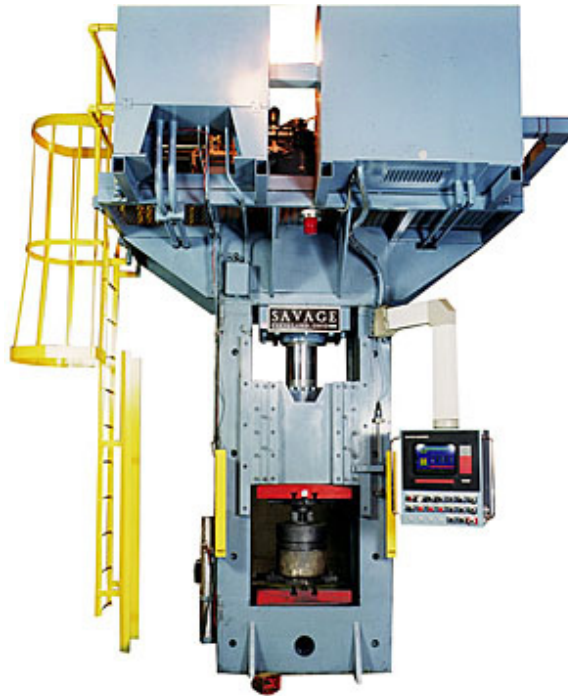
400 Ton Hot Extrusion Press to preform alloy steel prior to forging.
