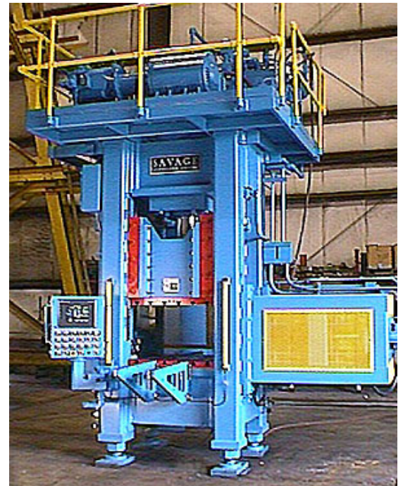
350 Ton Punch Press with barfeeder for 1 1/4" thick max. barstock.
