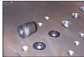
Spring Loaded Die Roller Bed for Small Die Sets
