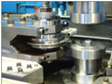
The opposing cutter and form roll assemblies are mounted on high-precision linear square rail slide assemblies. These are the zero clearance type typically used on grinders and CNC equipment. Each assembly has 2 linear rails with 4 slides to spread out the load and increase the stiffness. The 10" stroke per side allows pulleys from 2 3/8"Ø to a full 12"Ø.
