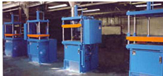
Programmable Laboratory Press designed for thermoplastic composite molding of medical implants
